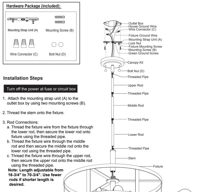
Thread the fixture wire through the canopy kit, then secure the rod assembly to the set threaded pipe of the canopy kit.
